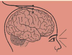
**In a BCI system,** the brain's electrical activity is detected through the scalp, from the surface of the brain, or from within the brain, and then processed by a computer to extract patterns indicating the user's intent. The patterns are then translated into commands for a device, such as moving a cursor on a computer screen or operating a wheelchair.
