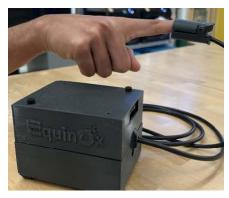
A team from Johns Hopkins University developed the EquinOx pulse oximeter to help correct skin tone biases in blood oxygen readings.
