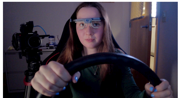
Eye-tracking glasses measure the number and duration of glances away from the roadway.
